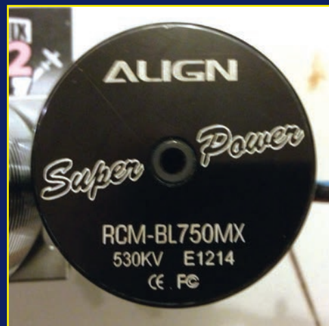
This is the 750MX which originally shipped with the 700E DFC, smaller all round than the 850MX
