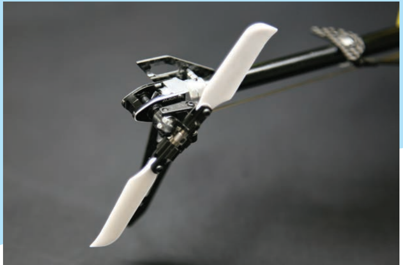
View of the new tail gear case and torque tube system
