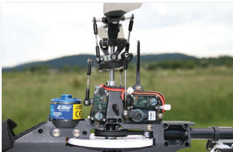
Brushless motor is forward mounted between the LiPo pack and rotor-head
