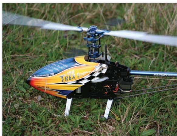
Because the swashplate had been trimmed and levelled on the bench, the very first hover was very stable
