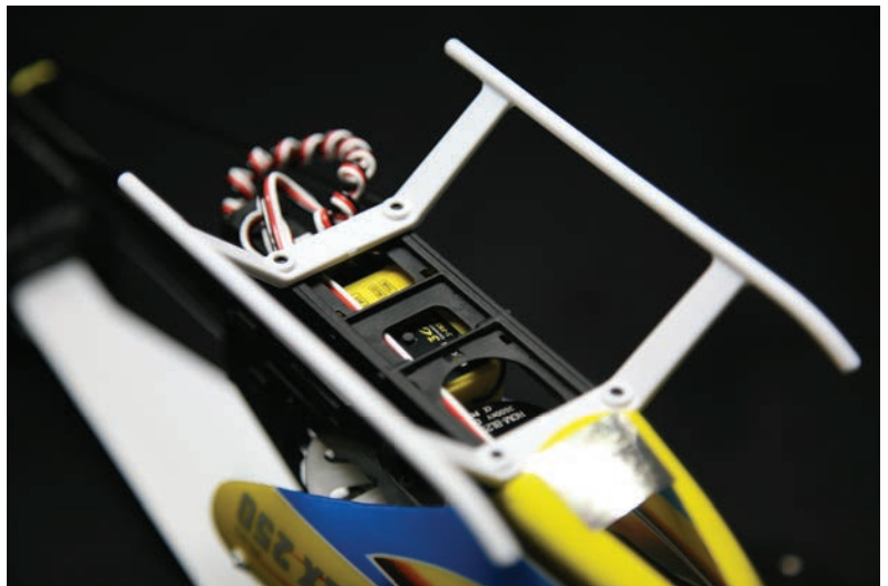
The 3GX MR flybarless system comes installed in the lower part of the frame
