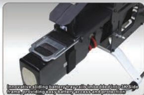
Innovative sliding battery tray is imbedded into the side frame, providing easy battery access and protection
