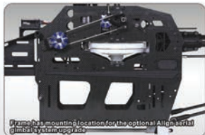
Frame has mounting location for the optional Align aerial gimbal system upgrade
