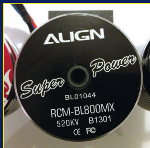
This is the 800MX for comparison. It is the same diameter as the 850 but a little lighter due to being slightly shorter. Note that it is a 520Kv so spins slower than the 850MX tested here
