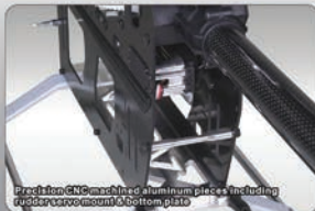
Precision CNC machined aluminum pieces including the servo mount & bottom plate
