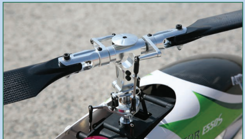
The look of the Raptor changes dramatically with the flybarless rotor, with the flybarless head you get a very nice and clean look of the mechanics
