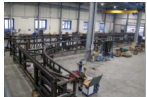
Track under construction at Gerstlauer factory in Germany for the pier's Iron Shark coaster
