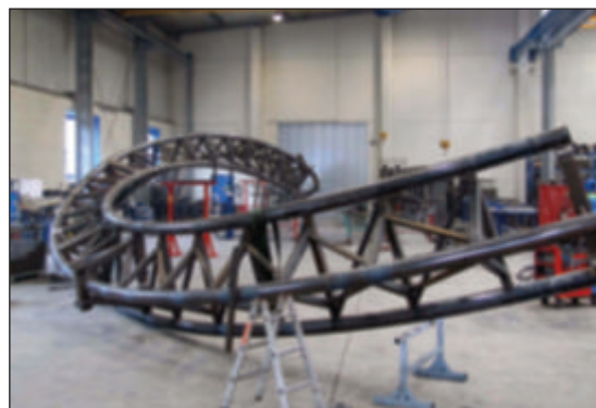
Track under construction at Gerstlauer factory in Germany for the pier's Iron Shark coaster
